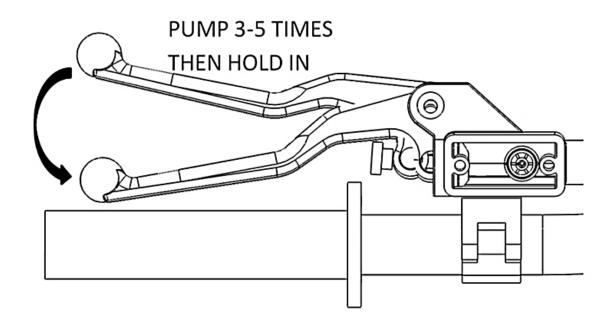
32. Using an 8mm wrench, open the bleed port. Air and fluid should come out of the bleed tube. Tighten the bleed port.
