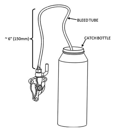
31. Pump the clutch lever 3-5 times then hold it against the bar/grip.
