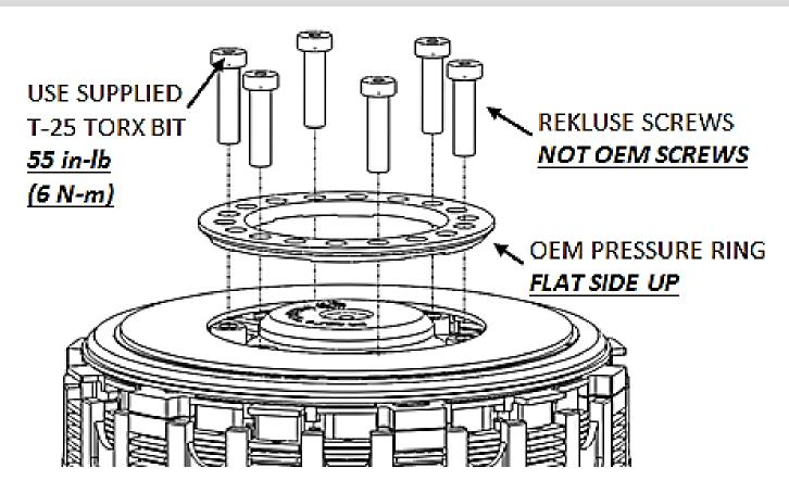
**NOTE:** There are 3 possible settings on the OEM Pressure Ring. Rekluse recommends setting II for all 4-strokes for optimum performance.
