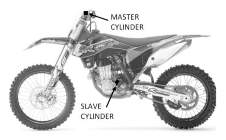
**NOTE:** Some 2017 FE450/501 slave cylinders have the banjo bleeder bolt and some have the straight fluid line. Follow the instructions based on the type of fluid line on your bike.
