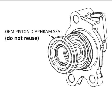
**NOTE:** When installing case sealing O-ring seal (OEM or Rekluse supplied) ensure it is seated against slave cylinder flange.
