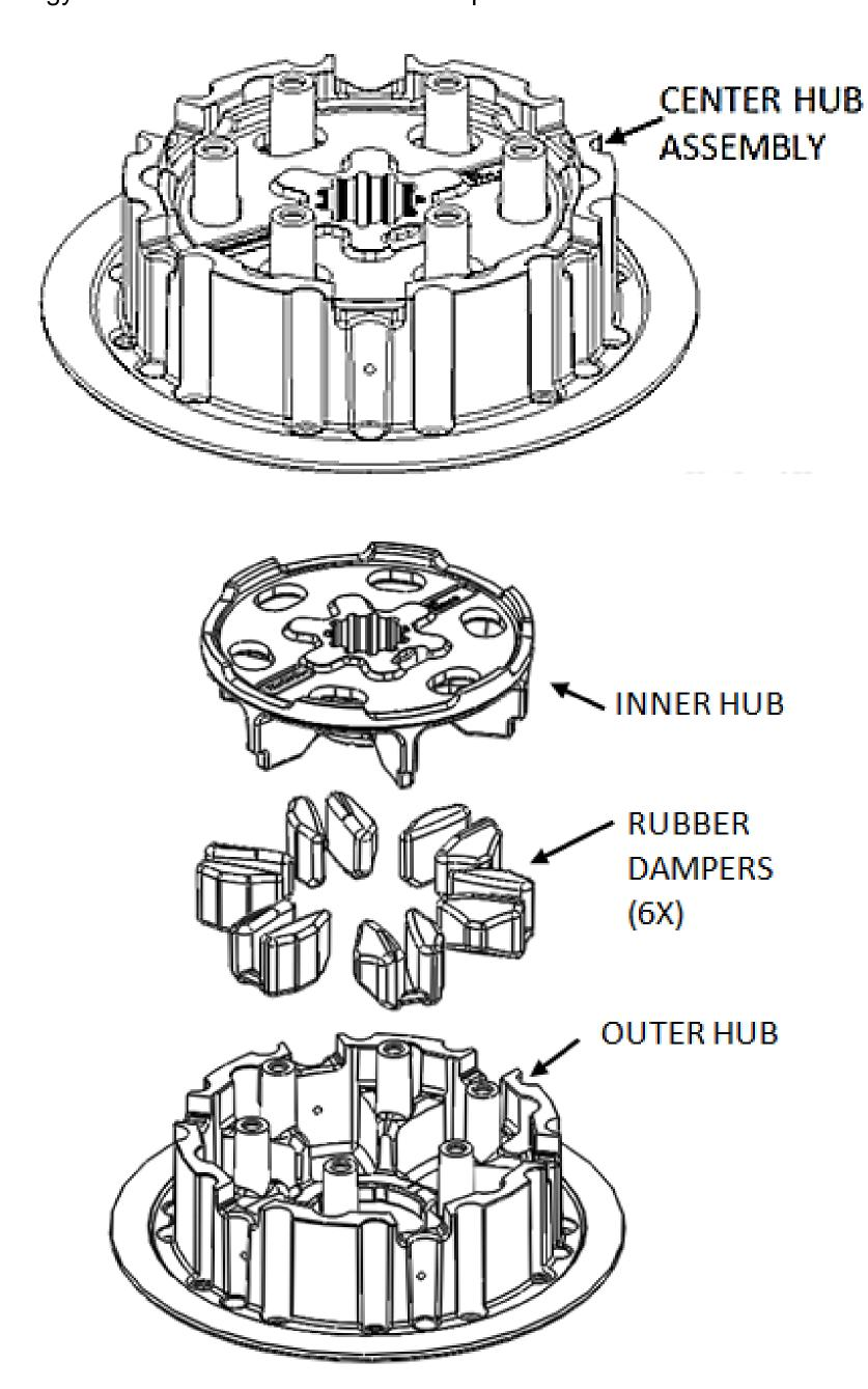
Over time, the rubber dampers will shrink due to heat and use. When this shrinkage occurs, the rotating action between the two hubs becomes loose or sloppy. This can cause hammering between the clutch parts which will reduce the life of the clutch.
