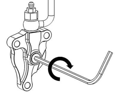
2.Once you have found the starting point, turn the adjuster clockwise 1 full turn plus 5 marks (or "1+5"). **This is NOT your final setting**, but it is a good reference point for using Free Play Gain to find the correct setting.
