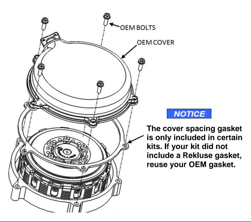
NOTE: If installing a Rekluse clutch cover, the spacing gasket is not needed.
