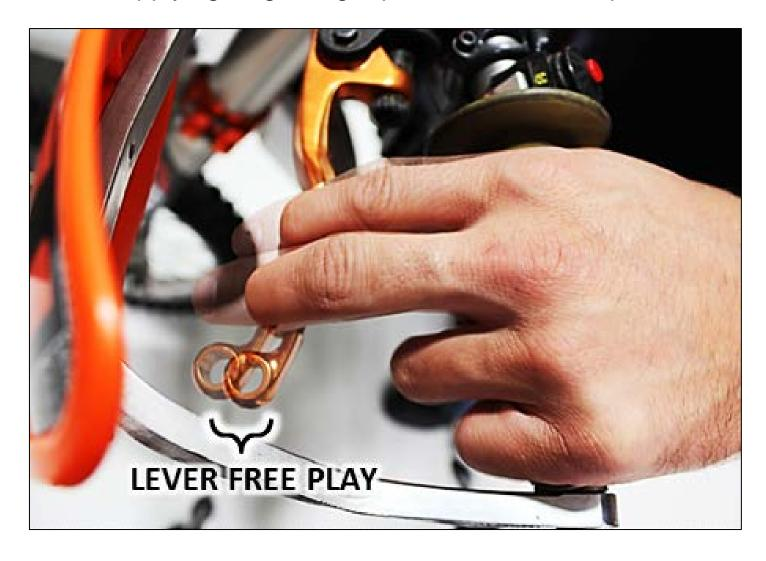
"Free Play Gain" is the increase of lever free play as the auto-clutch engages. This happens when the RPM increase from idle through around 5000 RPM. Free Play Gain is caused by the expansion of the EXP disk which lifts the pressure plate away from the throwout assembly.
