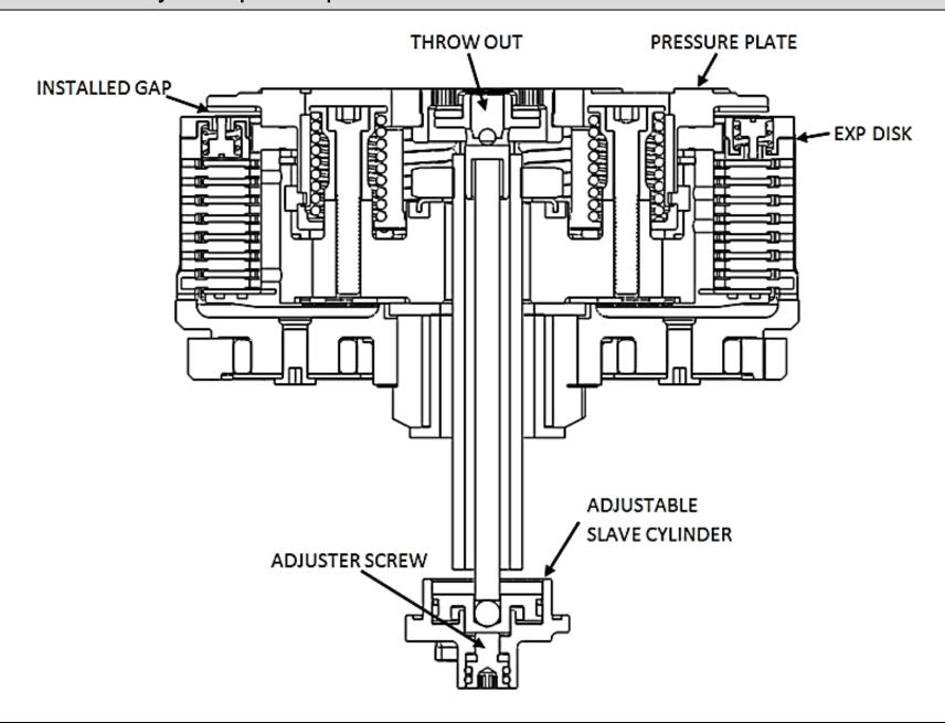
1. Using the long end of a 4mm Allen key, turn the adjuster screw clockwise until it stops under moderate pressure. You are trying to feel for the point at which the throwout will start to lift the pressure plate. This is the "starting point".
