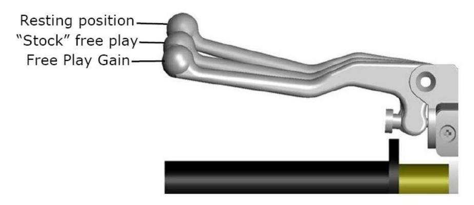
Optimal Free Play Gain yields **1/8-1/4**" **(3mm-6mm)** of clutch lever movement, measured at the end of the lever. This measurement at the lever correlates to achieving the ideal installed gap.
