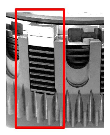
6. Hold a TEC drive plate so that the "shark fin" notches face toward the right. *All the drive plates will follow this orientation.*
