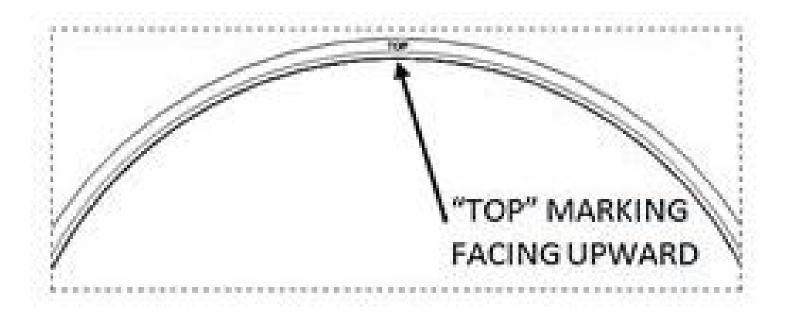
14. Place the OE Belleville spring onto the slider ring, with the rounded dome side facing up.
