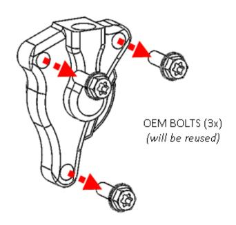
27. Mount the Rekluse slave cylinder to the engine using the OEM bolts.
